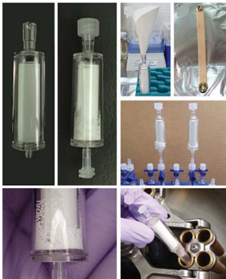
Fig. 2. Appearance of filter cartridges with a fluoroplastic membrane and work with them [23]
