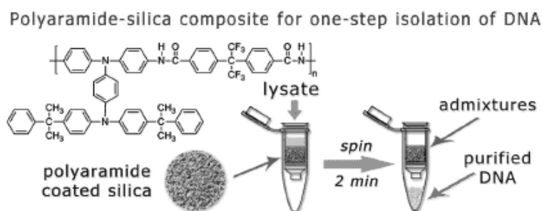
Fig. 3. Scheme of using the PAA–silica composite [46]
