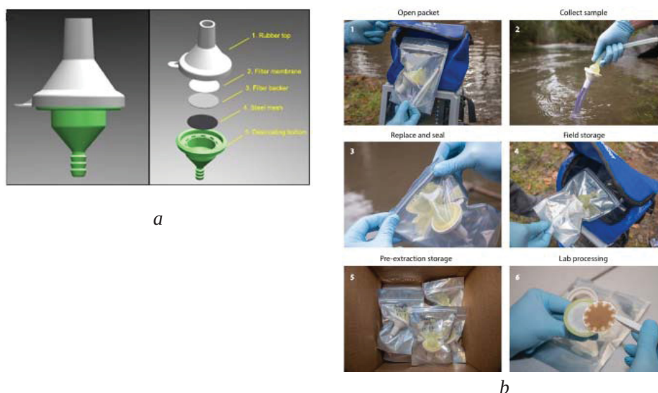
Fig.1. Appearance of a filter (a) with a PES membrane (b) and its use for water sampling [21]
